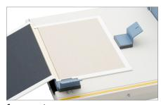
**Cover mounting** Covermounting is easy and quick with preglued end sheets and position magnets.
